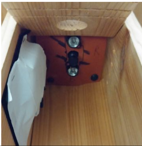
View inside the nestbox. Raspberry Pi computer attached to the side panel, camera and two infrared lights attached to the roof.
