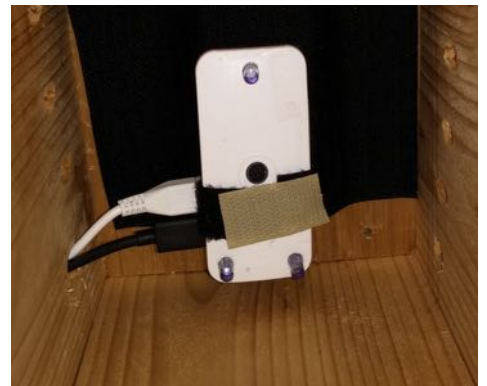
Raspberry pi computer in case with camera and lights. The case is fixed to the roof of the nest box with Velcro. The two cords, for power and Ethernet, run from the nest box into the house.
